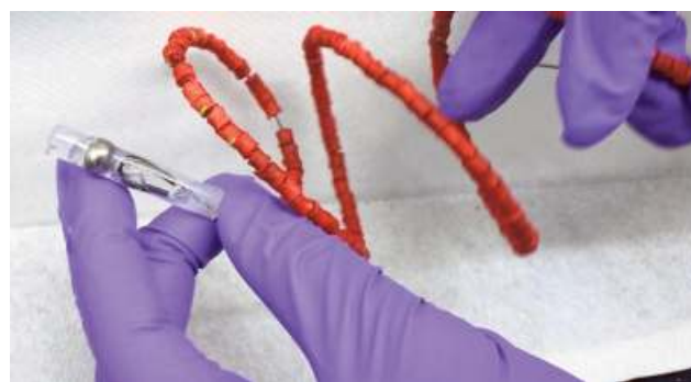
The researchers added 600 pills of different formulations to the coil made of a nickel-titanium alloy. ■ MALVIKA VERMA
