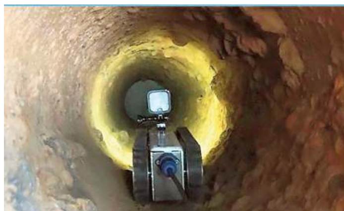
Mobile eye: The electrically-powered robot runs on four wheels connected using a conveyor belt and is tethered at one end.
