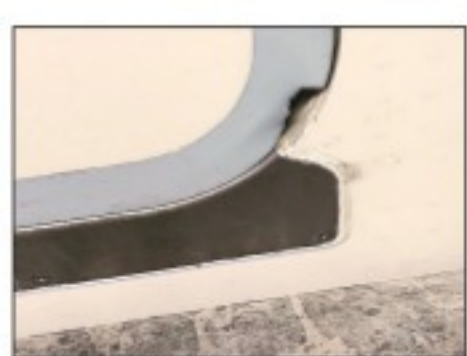
The crack on the Air India aircraft's door. ANI
