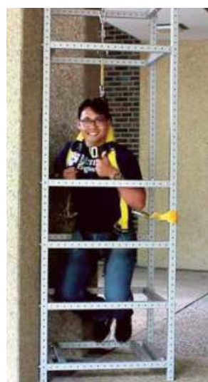
Firm grip: To demonstrate this, we used two 2-square-centimetre pieces of the adhesive to suspend me (85 kg) in the air, says Jolly. *SPECIAL ARRANGEMENT
