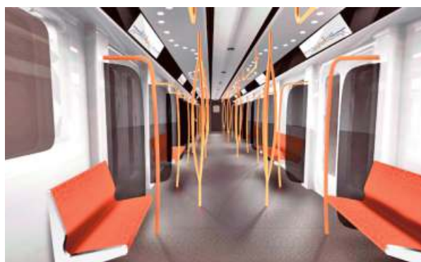
State-of-the-art: The coaches will be fully air-conditioned with humidity control, and have digital route and station display and international standard interiors. ■SPECIAL ARRANGEMENT
