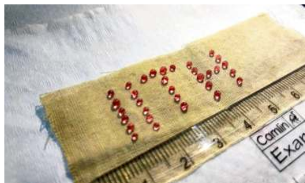
Waste no more: A simple process of particle distribution was used to achieve the two types of water-repelling.
