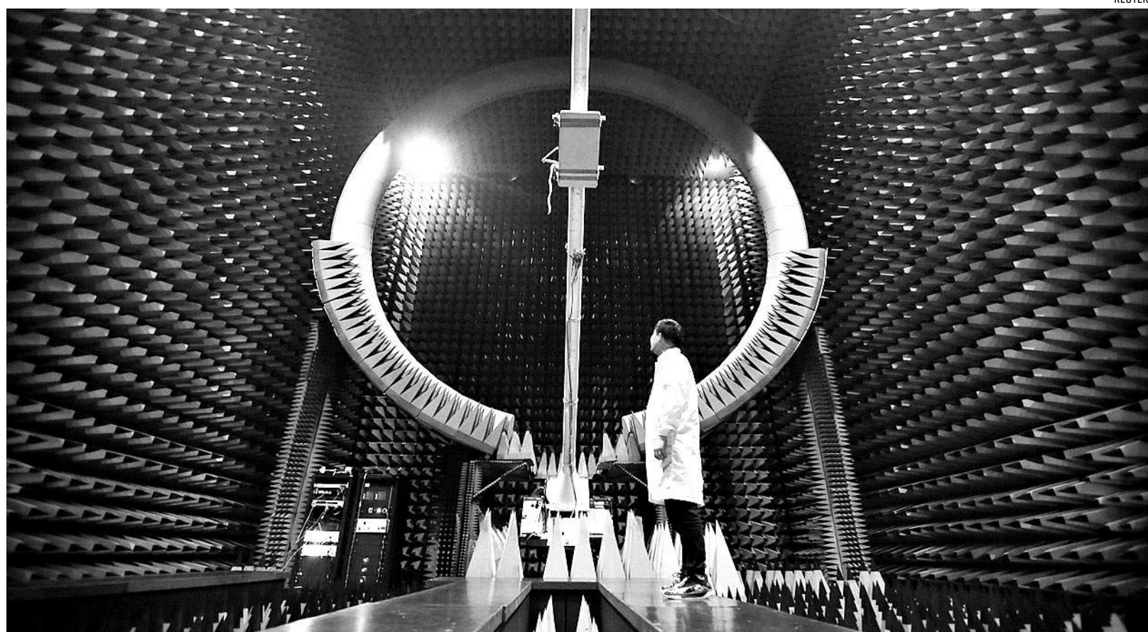
An engineer stands under a 5G base station antenna in Huawei's multi-probe spherical near-field testing system at its manufacturing centre in Guangdong, China
