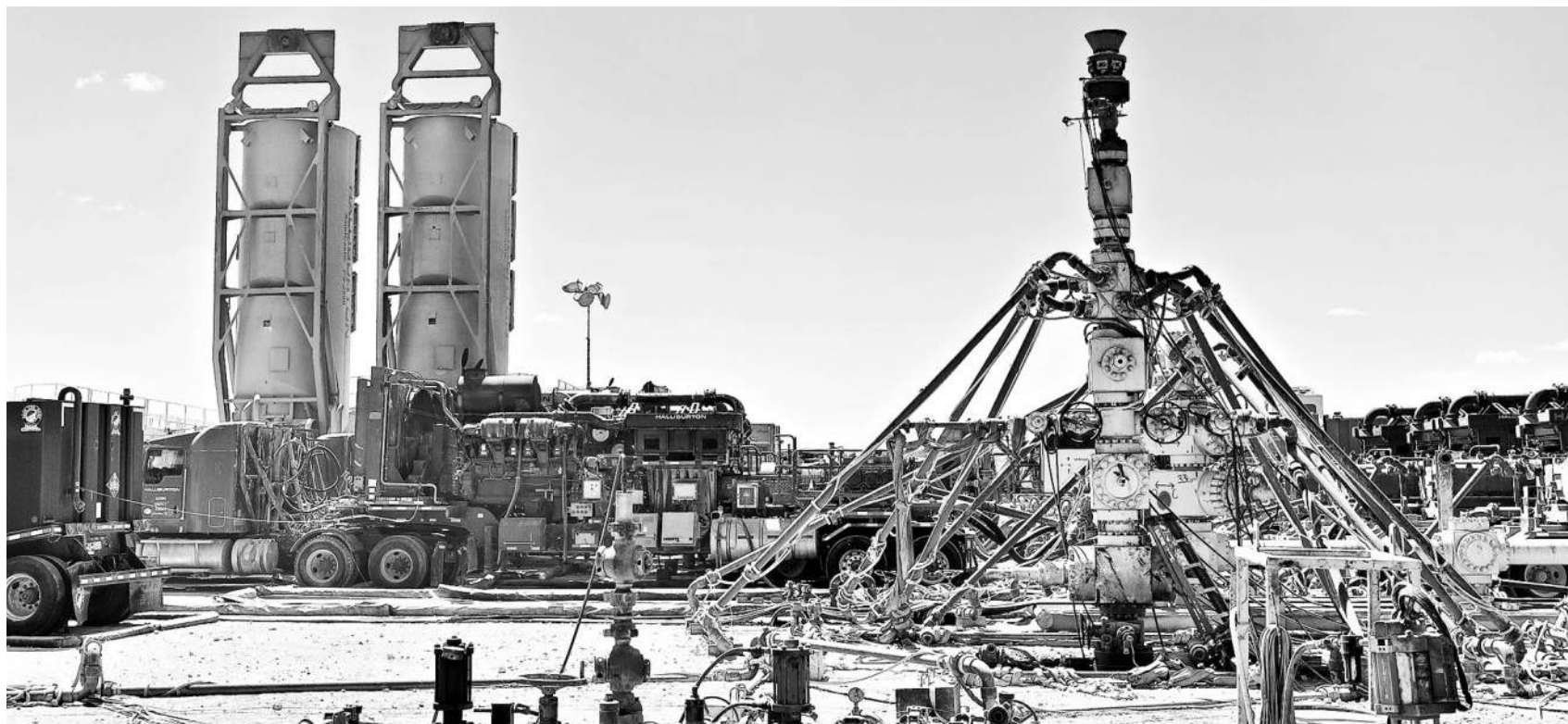
Unconventional oil: A wellhead on a fracking site leased by Oasis Petroleum in the Permian Basin oil production area near Wink, Texas
