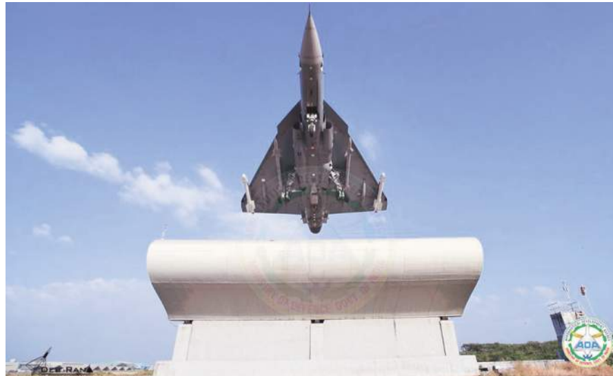
The Tejas prototype took off from the Navy's SBTF, but exactly as it would have from an aircraft carrier. Restraining gear locked the fighter's wheels as the engine revved up to maximum power
