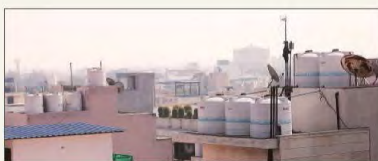
Many homes currently have underground reservoirs, from where water is pumped up to overhead tanks. Archive
