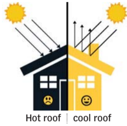
Hot roof | cool roof
