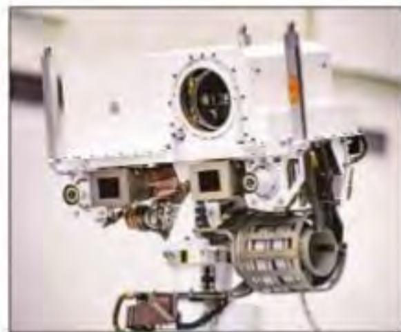
SuperCam that can vaporise rock material and study the resulting plasma. NASA/JPL-Caltech
