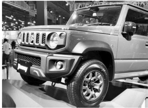
Maruti Suzuki showcased the 4th generation Japan model of off-road vehicle Jimny at the Auto Expo in Greater Noida. The vehicle, powered by a 1.5-litre petrol engine, has power of 75 kW/6,000 rpm and torque of 130 Nm/4,000 rpm PHOTO: TWITTER
