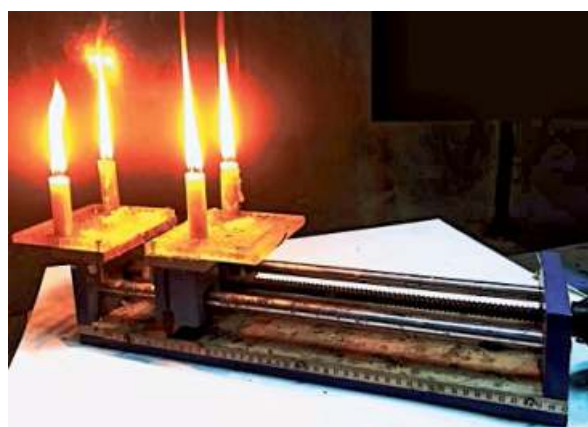
Synchronicity: The candle flames placed close together oscillate and show a rich variety of phenomena. • R.I. SUJITH
