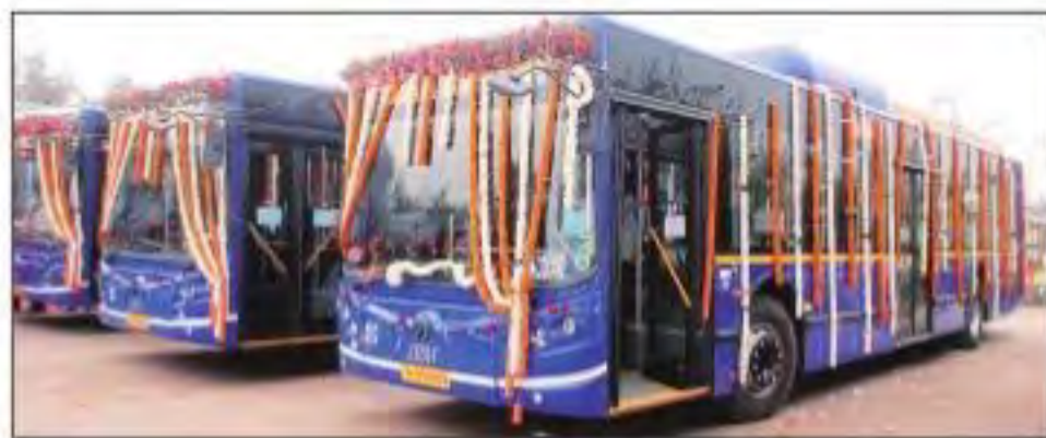
The new 37-seater buses are equipped with features such as GPS, fire detection systems, panic buttons and CCTV cameras
