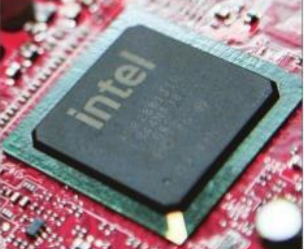
The new H range of Intel chips are made with 14-nanometer production technology. The company originally planned to upgrade to 10-nanometer in 2017, but that is only beginning to happen in mass volume this year
