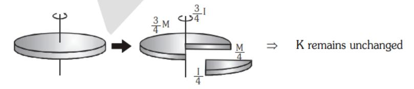
For Symmetrical attachment radius of gyration remains unchanged.
