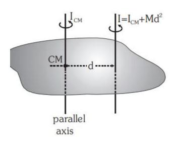
Statement: The moment of inertia of a body about an axis is equal to the sum of the moment of inertia of the body about a parallel axis passing through its centre of gravity and the product of its mass and the square of the distance between the two parallel axes.
